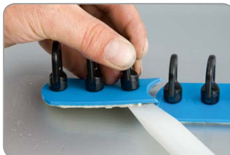
Remove the pad using the plastic wedge included in the kit.
