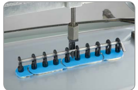
Use Line- or Strong-Puller to remove the panel deformation. Hold under tension and remove remaining tension in material with Alu-titanium hammers.
