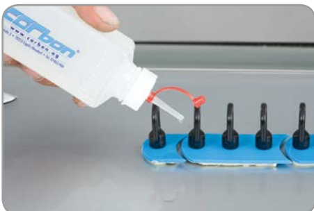
To loosen the pads put some cleaner on the outer area of the pads and let it soak in for some time.
