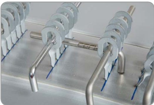
Arrangement of the bits on two edges with wider gaps
