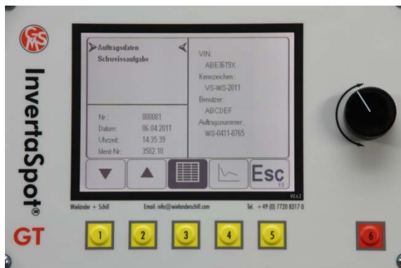
Button 3 will open the graphic display
