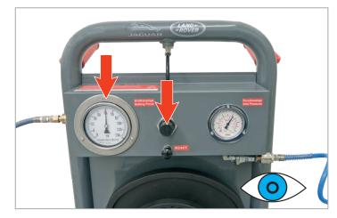
Connect the PowerPack to the spiral compressed air hose and connect the short-stroke cylinder SSC 40 for work.
