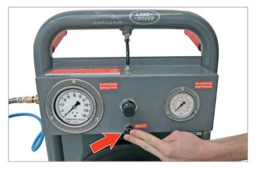
Empty air completely from tubular frame.
