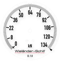
On all blind rivet adapters, the knob for the force display must be set to the maximum value of 78kN
