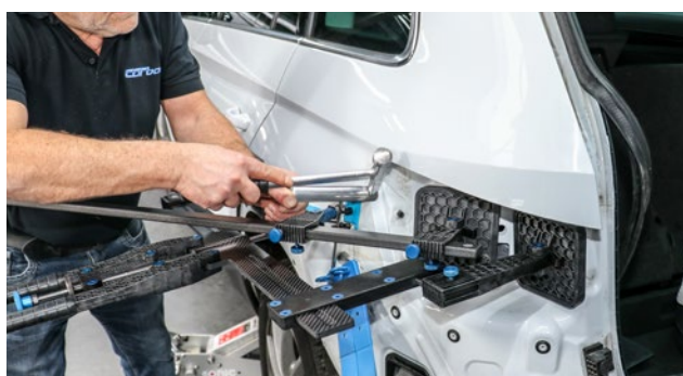
Insert with double foot when pressing
